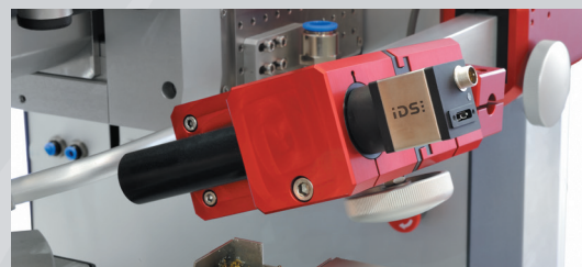
Side view camera, directly mounted on the frame
